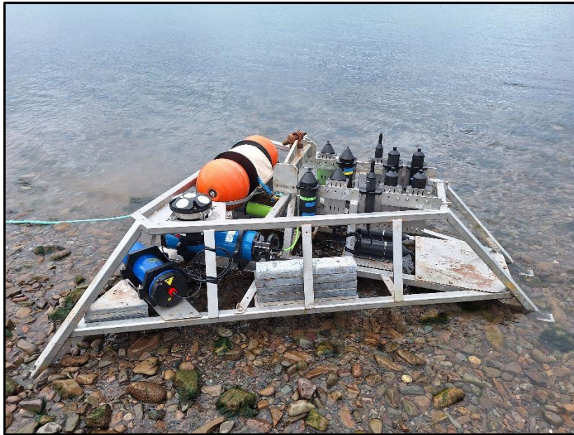
Figure 11: FAST-2 platform equipped with five Innovasea acoustic receiver technologies (with duplicates for redundancy), an ADCP and hydrophone for recording flow speed and underwater noise.
